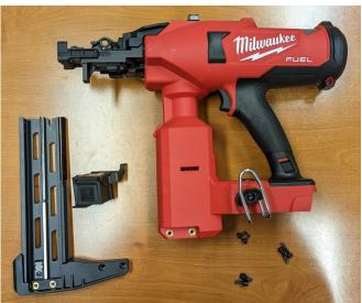
2. Save these bolts to reassembly the PowerDrive Enhanced Rail.
