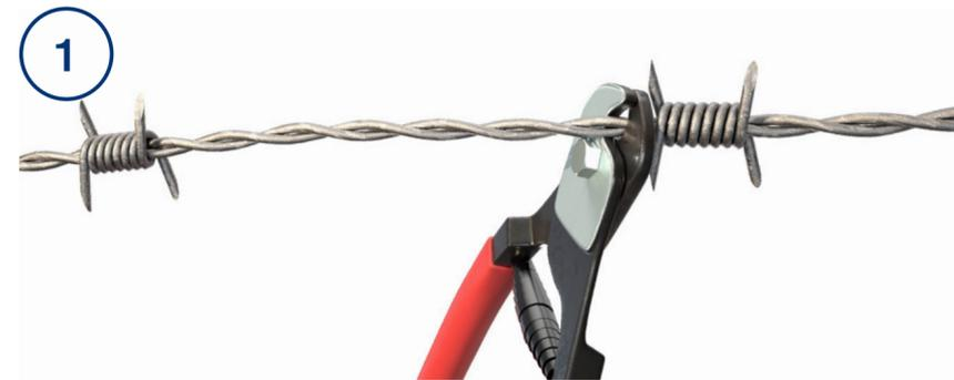
1 Cut wire at the barb, leaving at least 8 cm / 3 in of wire to make the join.
