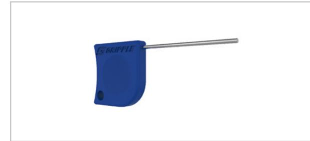
The Setting Key allows Gripple tensioners to be repositioned on the wire before tension is applied. To use, simply insert the key into the small hole adjacent to the main channel, releasing the roller and allowing the Gripple to move freely.
